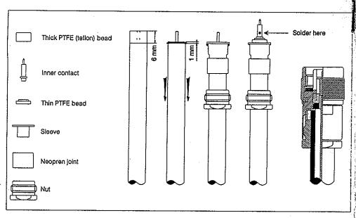
This connector can be used with cables RG213/U, H100, H500 or similar
