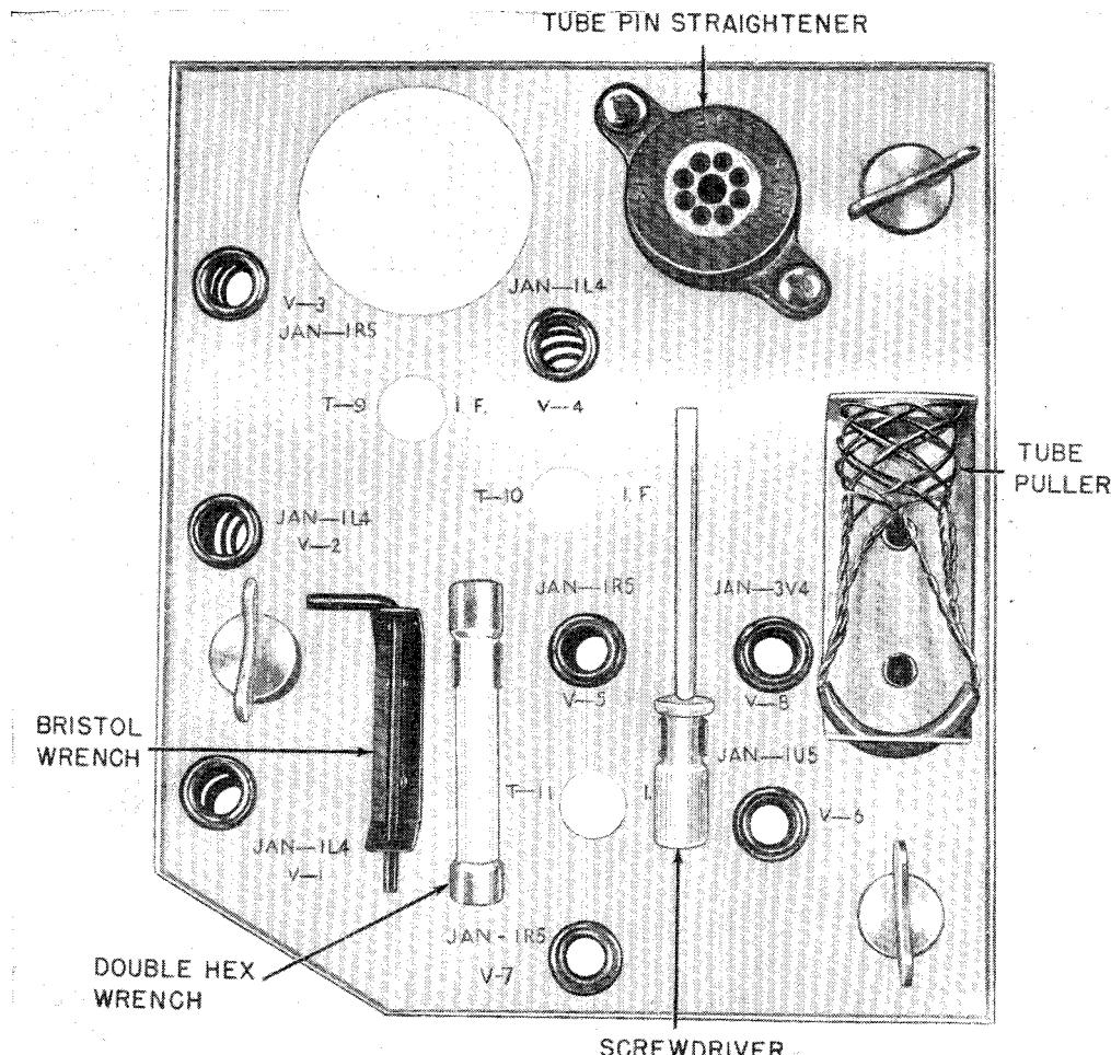
Figure 14. Radio Receiving Set AN/GRR-5, tools supplied.
