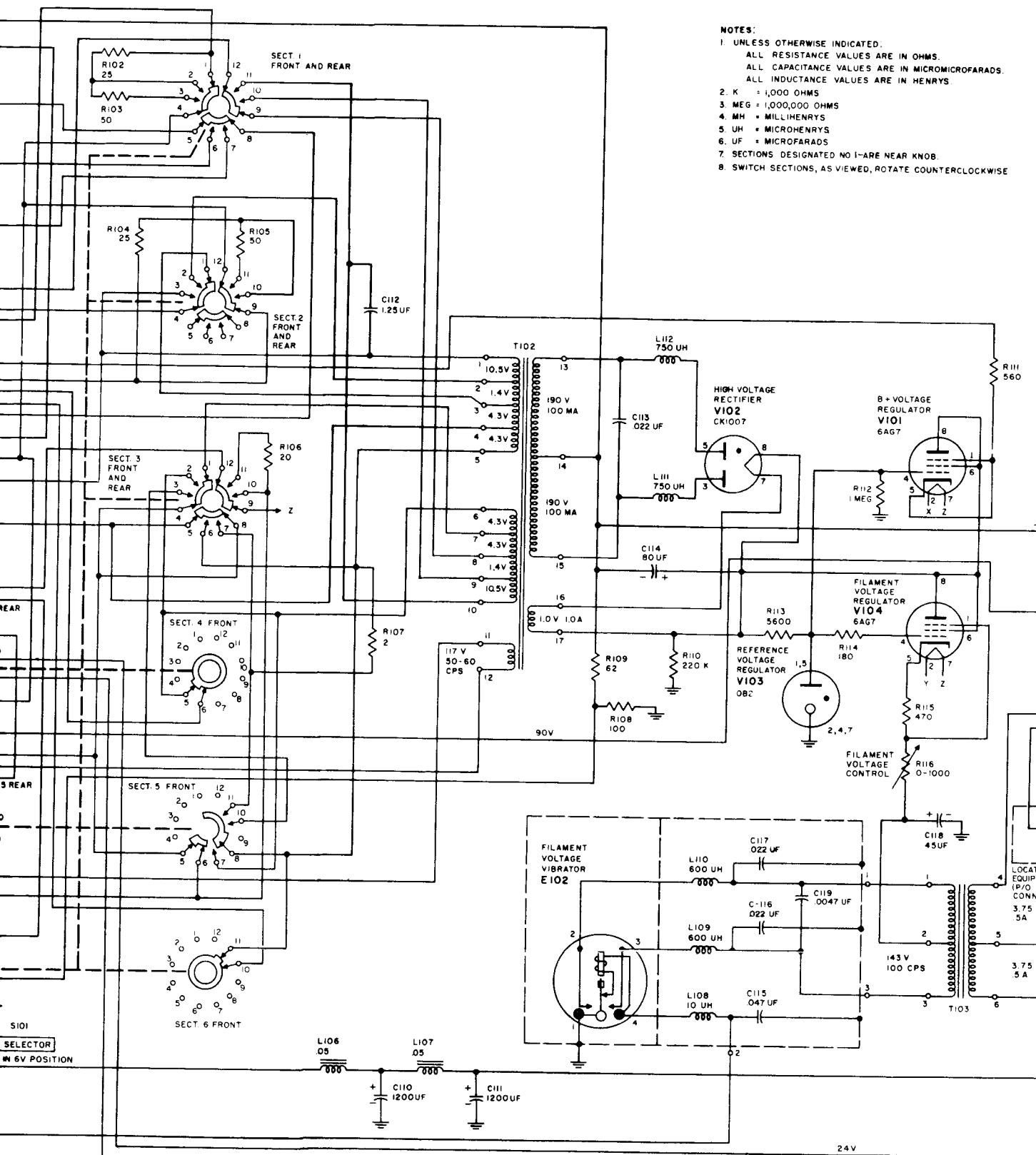
figure 47. Power Supply PP-308/URR, schematic diagram.
