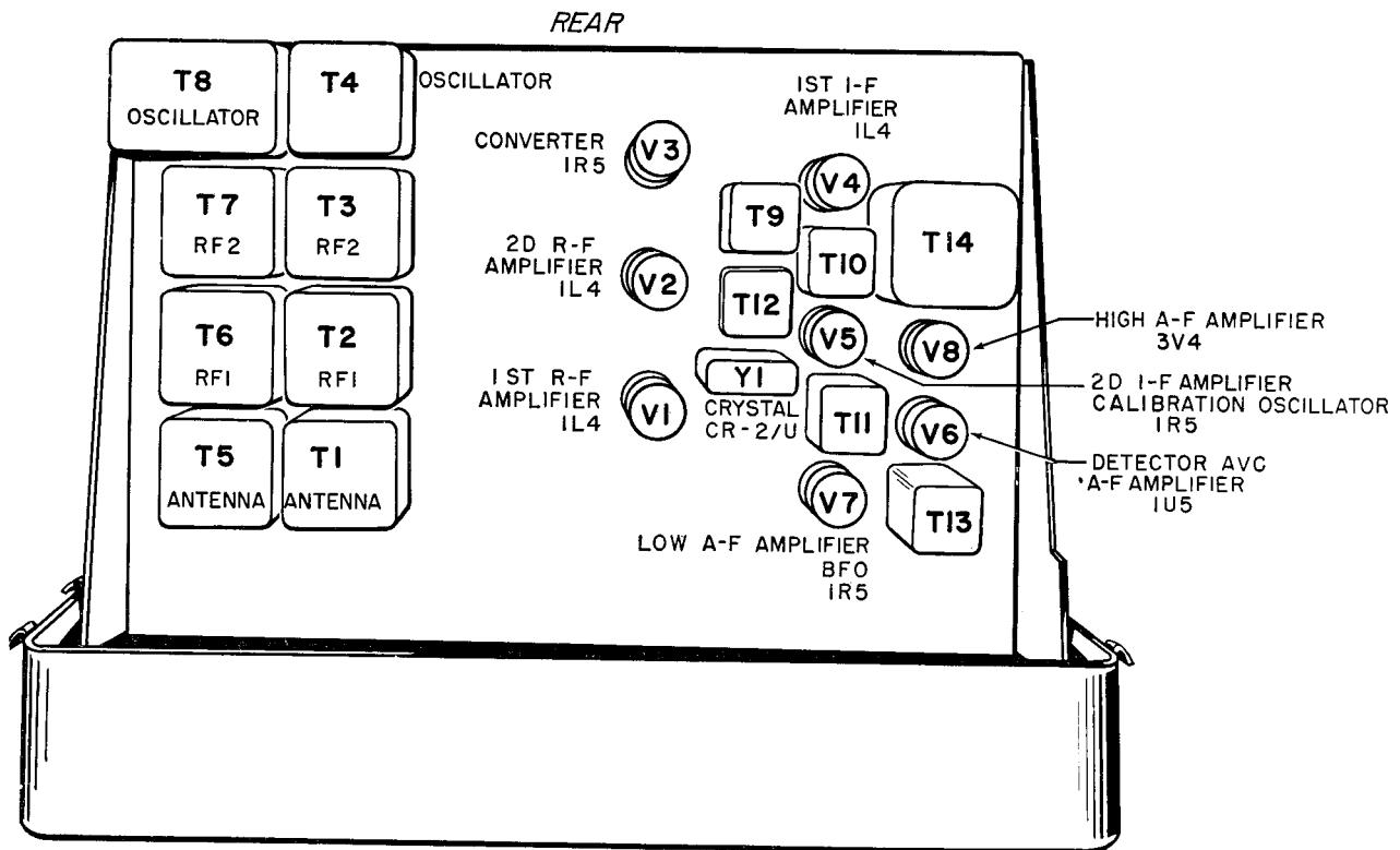
Figure 6. Radio Receiver R-174 URR, tube location.
