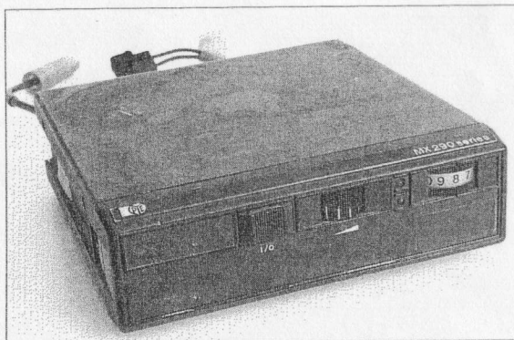
Top: The MX290 series is usually fitted with a 16-channel switch
