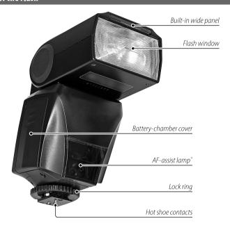
\* Lights to assist the focus operation if the shutter button is pressed halfway when lighting is poor. May not light with some cameras.
