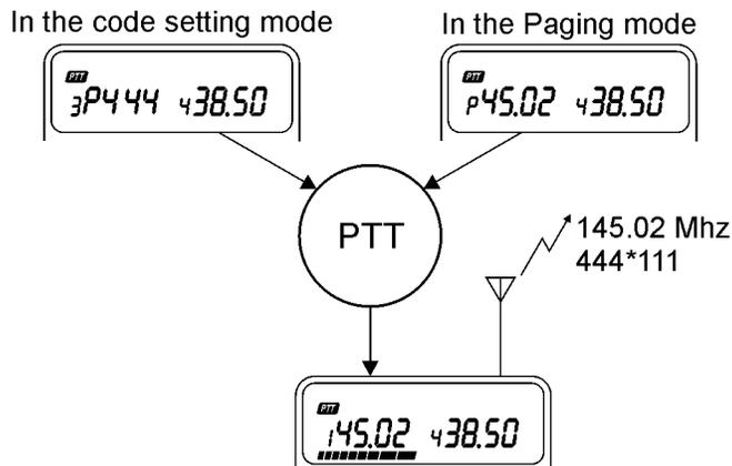
Local station code 444 and your station ID code are transmitted. The DTMF sounds as the codes are transmitted.
