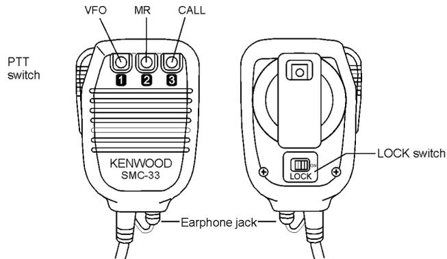
These keys function like the VFO, MR, and CALL keys on the front panel of the transceiver.
