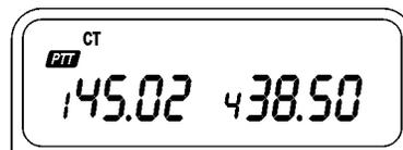
The desired band will now operate in the Tone Squelch mode. That is, squelch will not open until the selected tone is received as a portion of the incoming signal.
