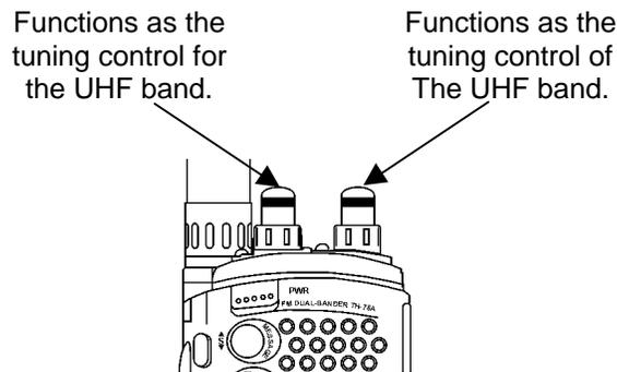
The inside knob of the LEFT control functions as the TUNING control for the VHF band, and the inside knob of the RIGHT control functions as the TUNING control for the UHF band.
