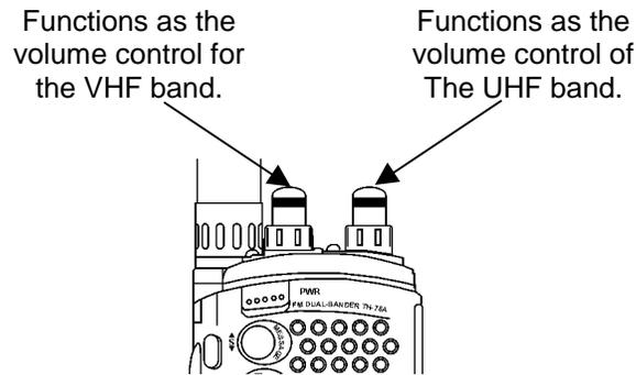
The inside knob of the LEFT control functions as the VOLUME control for the VHF band, and the inside knob of the RIGHT control functions as the VOLUME control for the UHF band.
