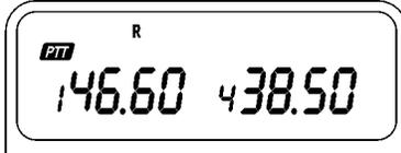
Press the **F** key, then press the **SHIFT/REV** key again to return to normal. The R indicator will disappear.
