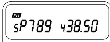
Press the PTT switch. Communication is possible in both the Paging and code setting mode.
