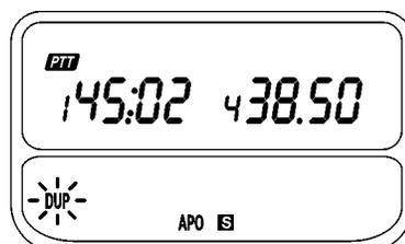
In this mode, the microphone sensitivity and receive audio are reduced automatically to prevent howling. The transmitter output power is also automatically set to the **EL** position. You can select the desired transmitter output power by pressing the **F** key, then pressing the **D/LOW** key.
