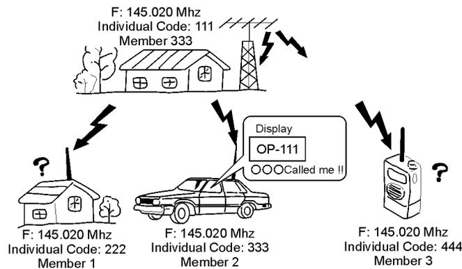
You should determine the common group paging code and individual codes in advance. You can enter three-digit codes from 000 to 999.
