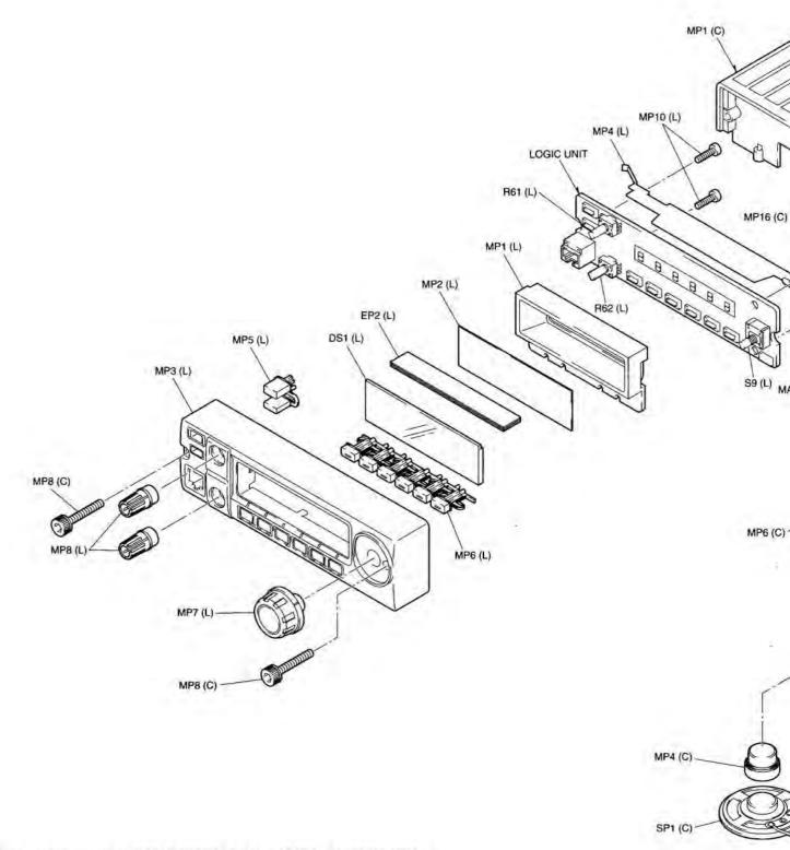
UNIT abbreviation (C): CHASSIS PARTS, (L): LOGIC UNIT, (M): MAIN UNIT
