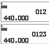
If no DTMF code is stored in the selected channel, the frequency display is restored.
