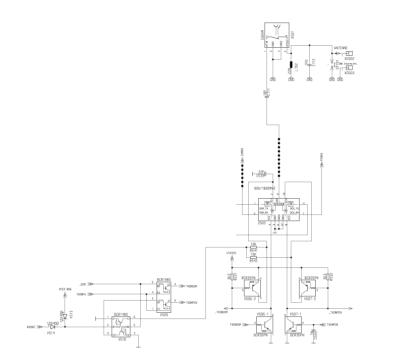
b: The electrical antenna switch (Diplexer Z503) for the differentiation between the receiving and transmitting signals, just like the differentiation between GSM900 and GSM1800 To do so the signals "\_GSM; TXONPA; RXON2" are required to switch the
