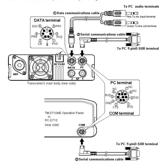
Data communications cable (for audio in/out) pin configuration
