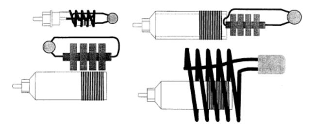
Once a dip is found the coupling coil and the inductor of the circuit under test should be separated until the dip is barely evident. The frequency should be read at this point for maximum accuracy.
