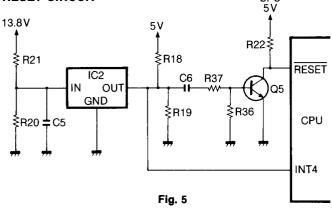
RESET port remains "HIGH" except when the CPU is reset. The following is a diagram for the reset circuit and timing chart.
