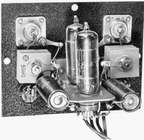
Fig. 4—Components of Dioplex mounted in space-saving arrangement
