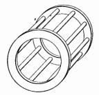
Fig. 18-3. Winding on Squirrel-Cage Rotor
