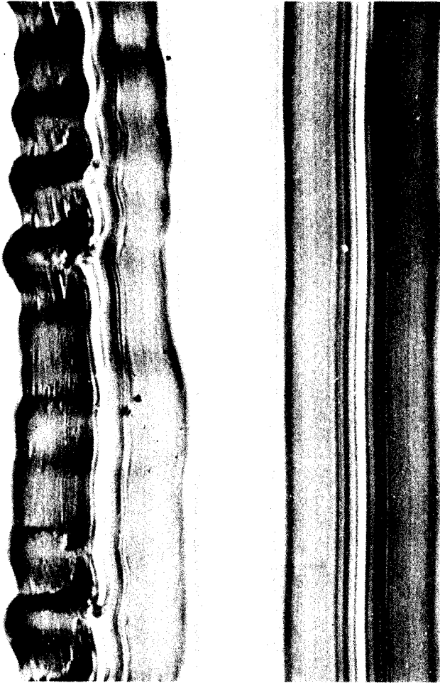
FIG. R/17. Heavily modulated groove after 165 playings showing slight signs of damage. Mag. 300x.
