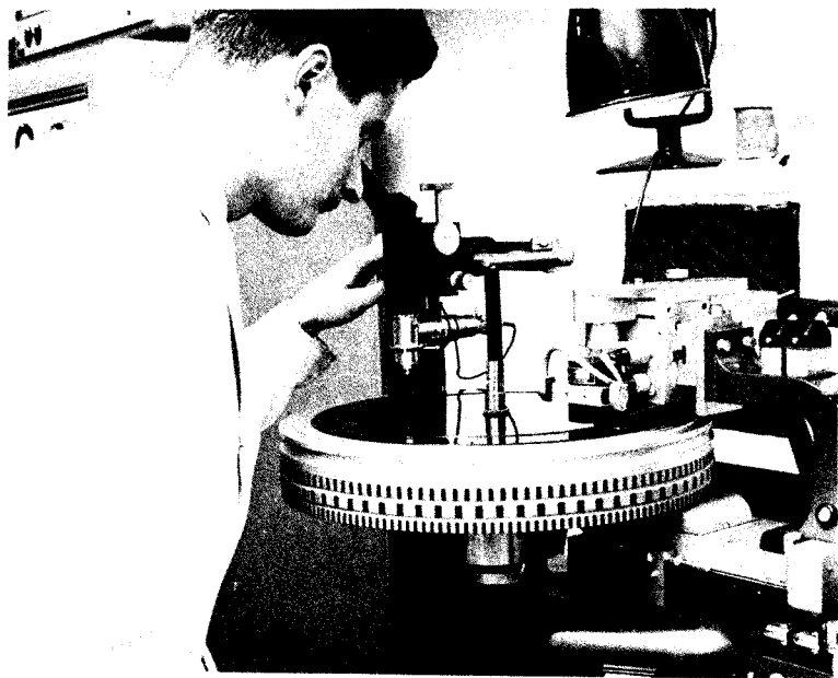
FIG. R/10. Keen observation of process of cutting lacquer disc at Decca studios. Note swarf extraction plant in right-hand background.
