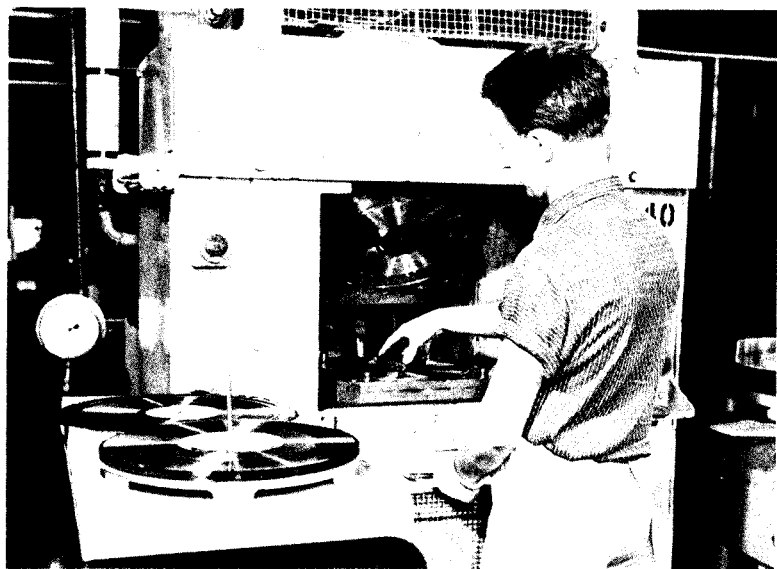
FIG. R/13. Pressing the final record.
