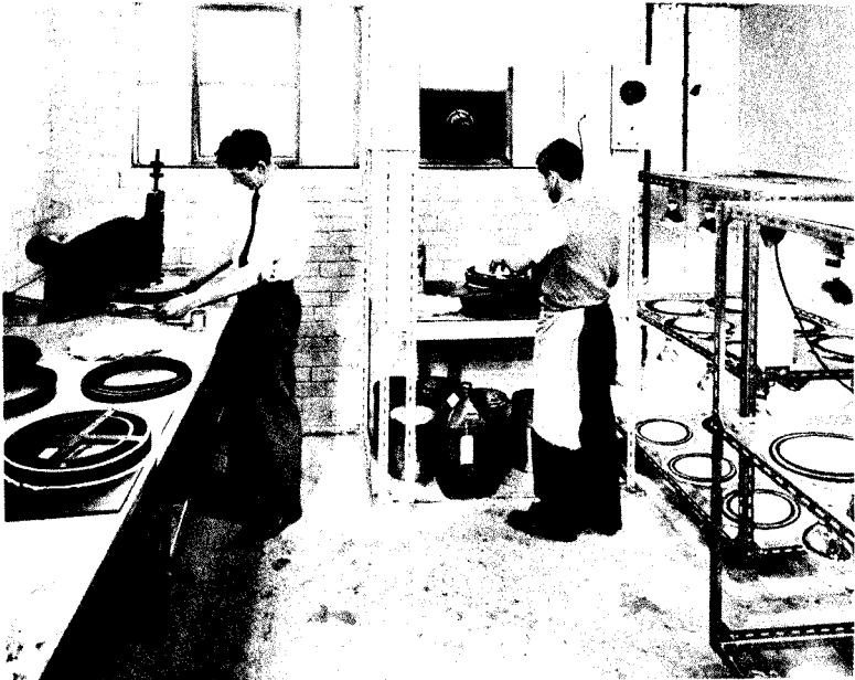
FIG. R/19A. Small plant devoted to the production of roll surrounds.
