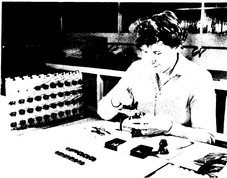
FIG. P/7. Mounting armature in Decca pickup head. Note fine connecting leads on right.
