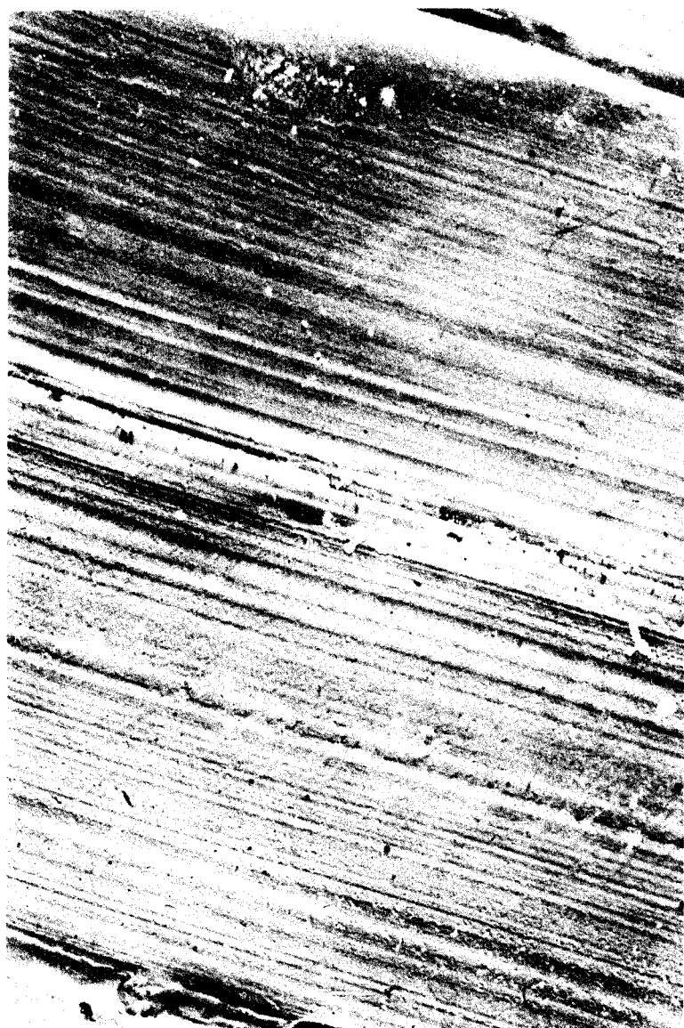
FIG. E/6A. Part of unplayed microgroove as revealed by Electron Microscope. Side view. Mag. 3,000x.
